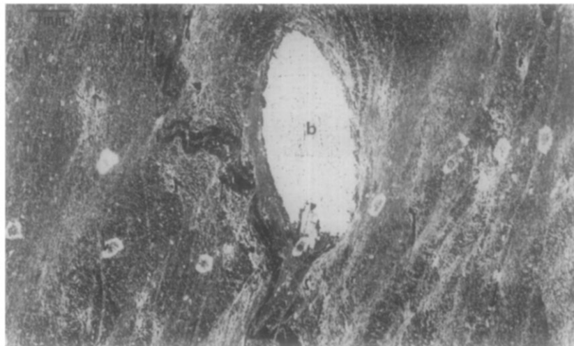
Fig. 9. Advanced stage microshears at < 45^\circ (thin bands) and > 45^\circ (wide bands) to S_1 . The former may be attenuated or deflected (bottom left) or cut straight across the latter (right). Note the mild differentiation into mica rich and quartz rich zones, the latter forming the intershear spaces. b—biotite. S_1 slopes towards bottom right. (Reverse contact print.)
